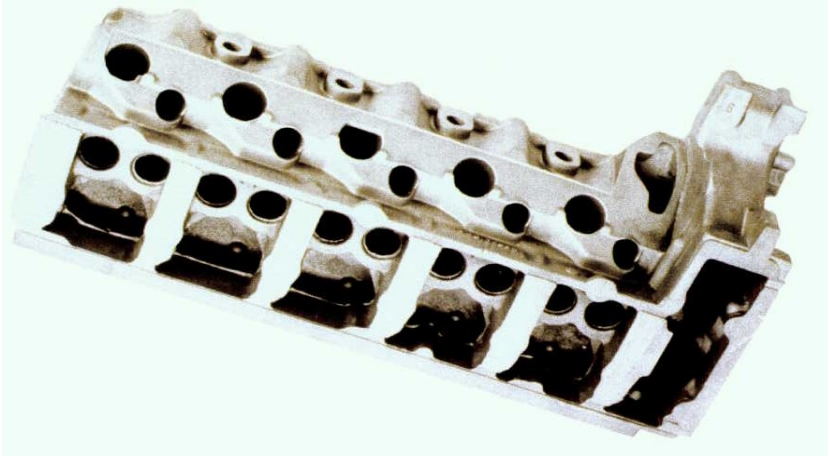
Fig. 1. The experimental cylinder head casting
