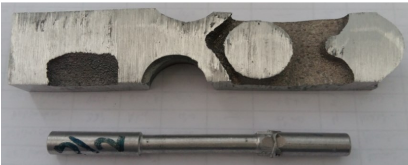
Fig. 2. Part of casting and sample for tensile test
